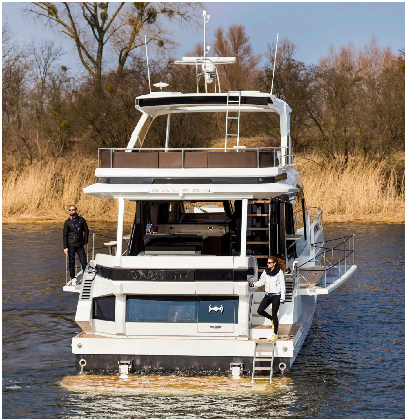
Hydraulic platform and access to the crew cabin
